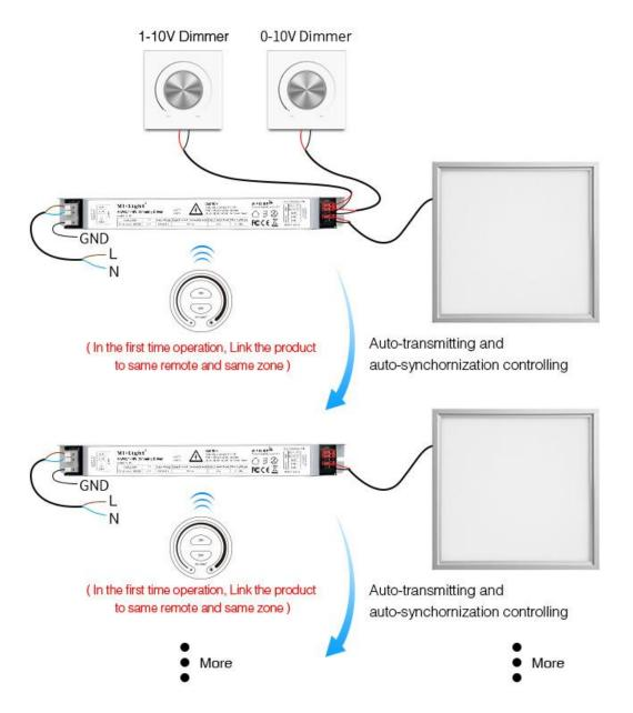
**Note:** If you need the 0/1~1V dimming panel to control many controllers at the same time, you must use same remote and same zone to link the controller. Controller just transmit the signal from the first time operation linked by remote (The signal is first signal); if you want to change, you need to unlink the first signal, then use another remote to link it (this signal is the first signal from remote), so when you want to change, please unlink the first signal, then link to another.
